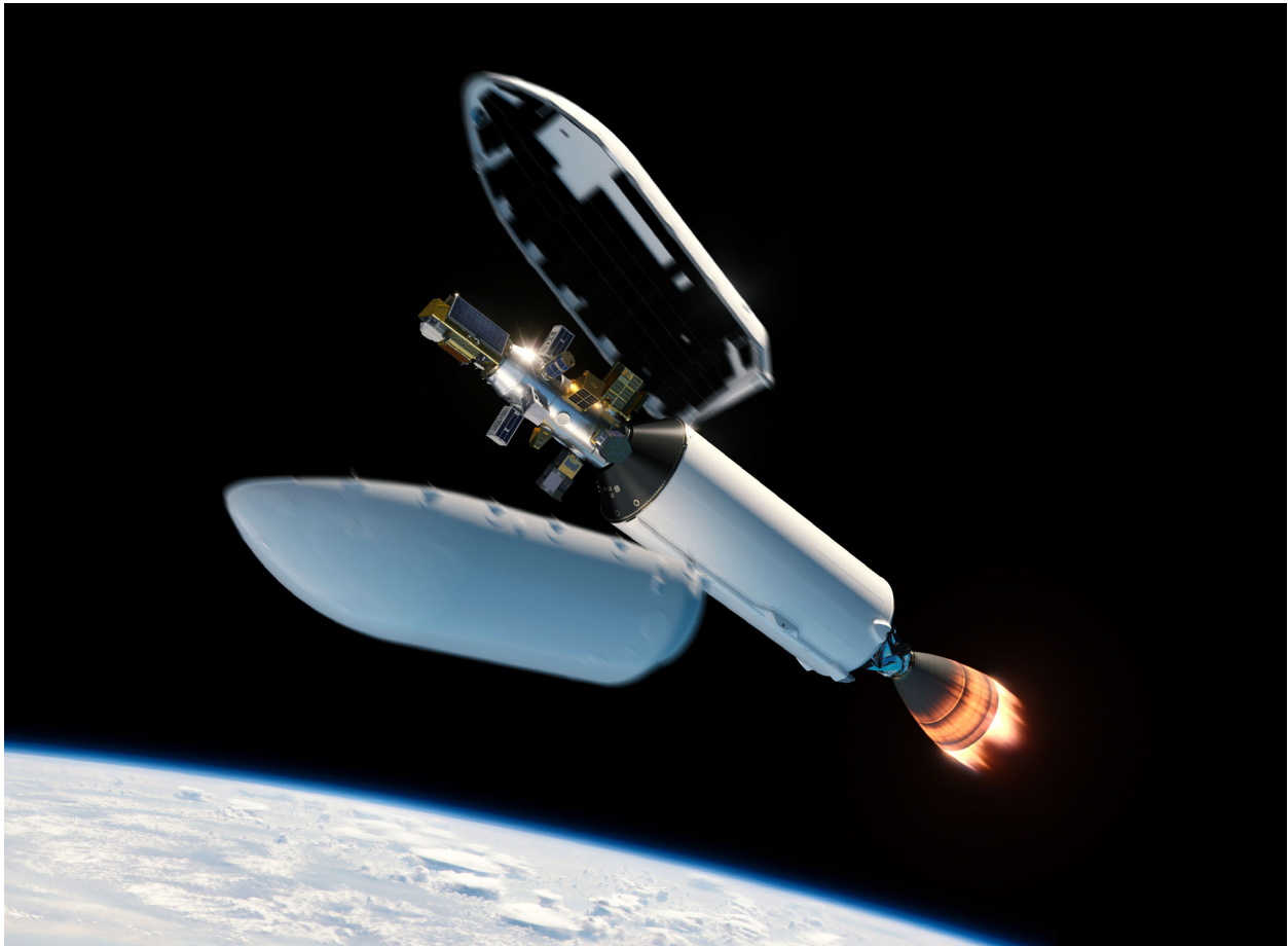
Figure 1-1: Example Mission Configuration using Rideshare Dispenser Rings
