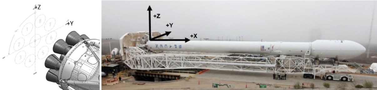
Figure 4-1: Launch Vehicle Coordinate Frame
